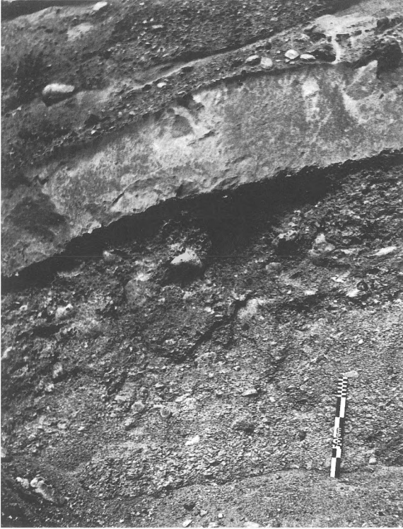
Figure 6. Detail of right-hand section in Figure 5. Note the grain-size contrast between the fluvially reworked, bedded diamictic gravel (bottom part) and the massive flowtill (top part). The scale is 0.5 m long.
