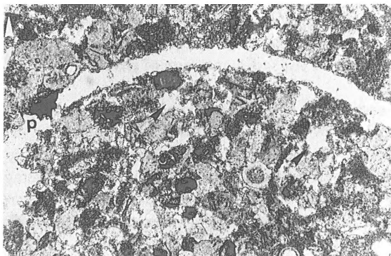
Figure 26. CV M – Muddy calcisiltite with few, slightly dissolution-enlarged pores, probably coinciding with moulds of dissolved (aragonitic, high Mg-calcitic) clasts (arrows). Large (early-diagenetic) mouldic pore, locally filled with early-diagenetic pyrite (p) after dissolution of pelecypod shell. Common (poorly visible) equant, fine-crystalline cement. Width of view = 1.4 mm.
