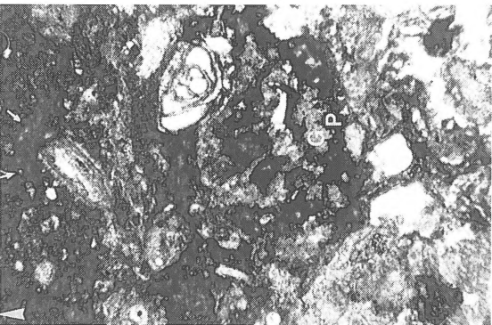
Figure 11. GRB 1 – Boundary between coarse-grained calcarenite and calcilutite (A clay). The bioclasts of the calcarenite have been mineralised by glauconite (G) and pyrite (P). Bioclasts and matrix have been partly dissolved. The calcarenite is covered by a layer of smectitic calcilutite with peloids and bioclasts. This wackestone has been pyritised at the basis and consists upwards of calcilutite laminae that drape conformably over extruding bioclasts (small arrows). Top is at left (large arrow). Width of view = 1.4 mm.
