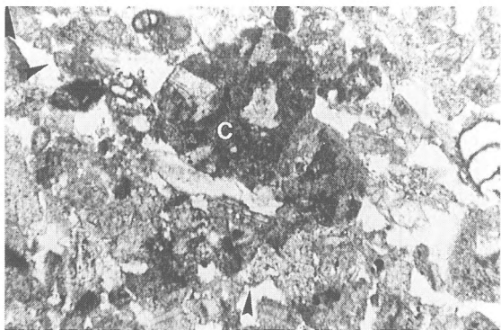
Figure 23. CU 4 – Porous, medium- and fine-grained calcarenite with (non-oxidised) glauconitised and pyritised intraclast (C) and dissolution-enlarged pores of which the margins are lined by (iron-hydroxide) clay minerals, suggesting early dissolution before clay-mineral genesis (arrows). Width of view = 1.4 mm.
