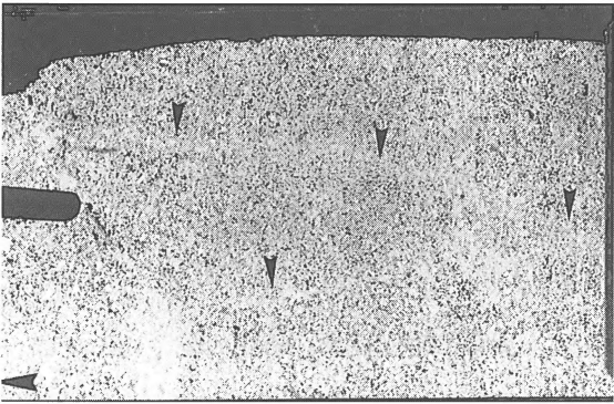
Figure 15. GRA 7 (height 4 cm, top is at left) – Muddy, medium- to fine-grained, laminated calcarenite with traces of bioturbation (arrows).
