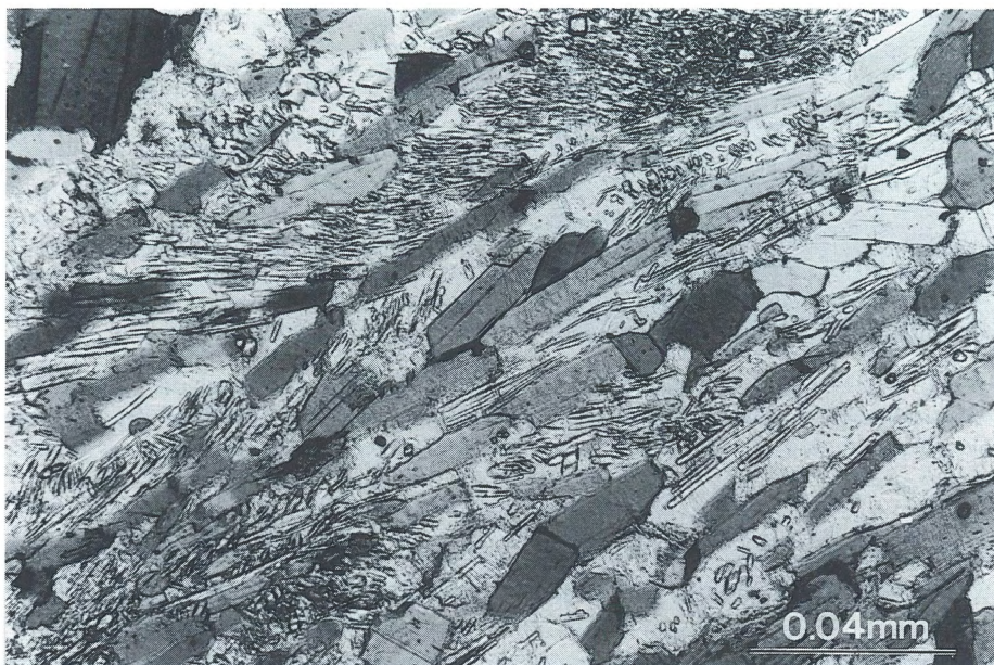
Photograph 1. Intensely folded S1 planes defined by polygonized sillimanite in a schist. S2 minerals (biotite and sillimanite) show parallel arrangement and tend to follow the axial-plane direction of the folds. Both biotite and sillimanite are included in a large cordierite porphyroblast.
