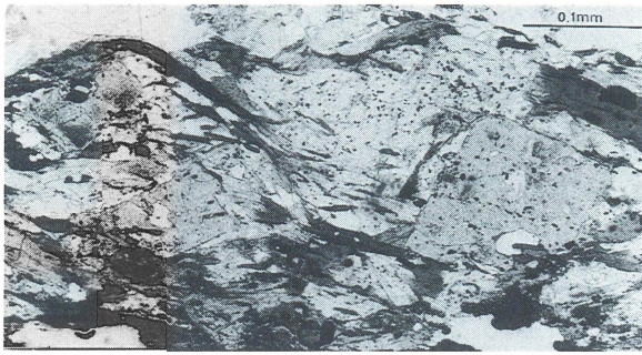
Photograph 2. Warped S2 foliation flattened by late folding phases around post-kinematic andalusite porphyroblasts. Andalusite is idioblastic and includes small ilmenite crystals parallel to the foliation. Note the asymmetry of the flattening, the pressure-shadows and the andalusite porphyroblasts, which are broken at the contacts with unprotected areas. Pressure-shadows are filled by plagioclase, quartz and biotite.
