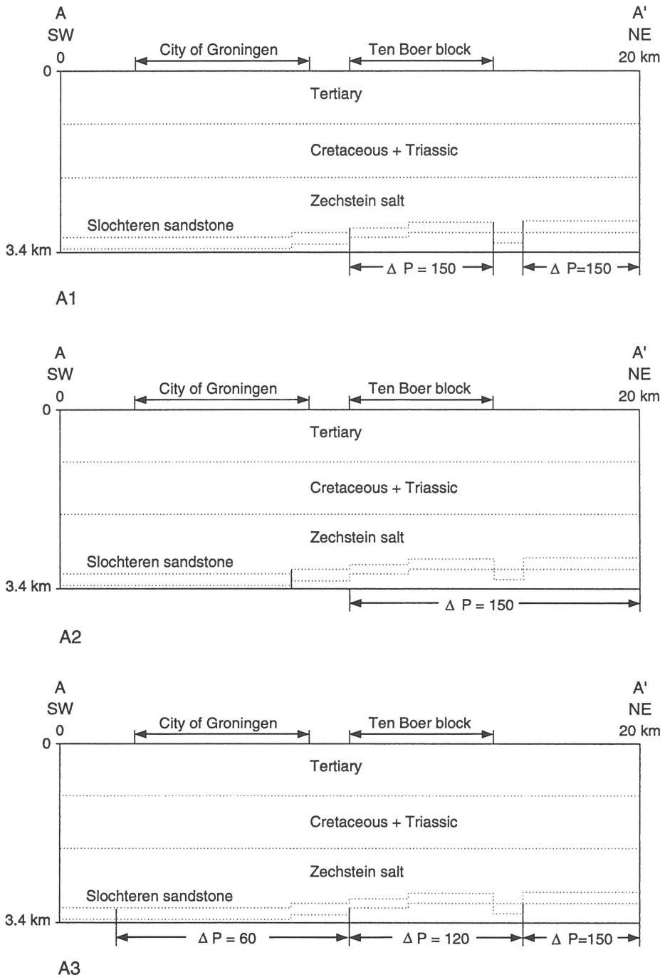
Fig. 3. GEOFEP finite-element study for SW-NE section A-A'. Pressure drop ( \Delta P in bar), in model A1 to A3.
