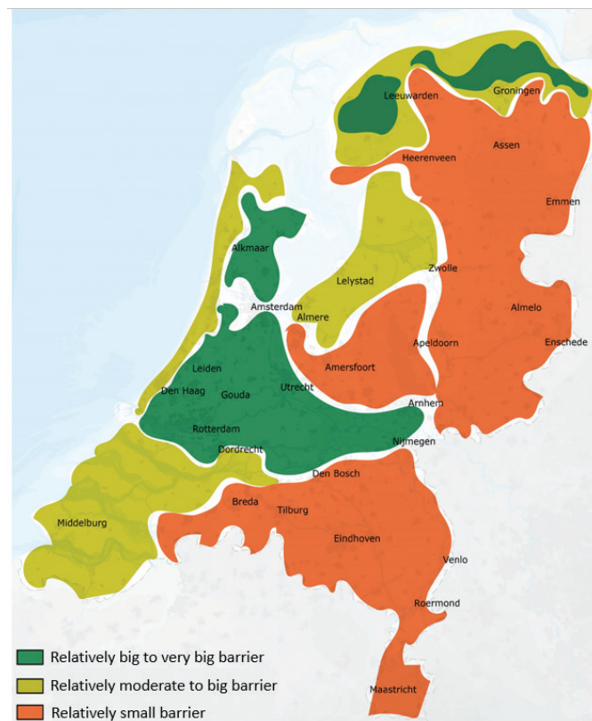
Figure 9. Spatial distribution of natural barriers to groundwater contamination (from Hendriks et al., 2023), based on thickness of first separating layer; pyrite content at 10 m-mv and self-cleaning capacity in the top layer of the subsurface.
