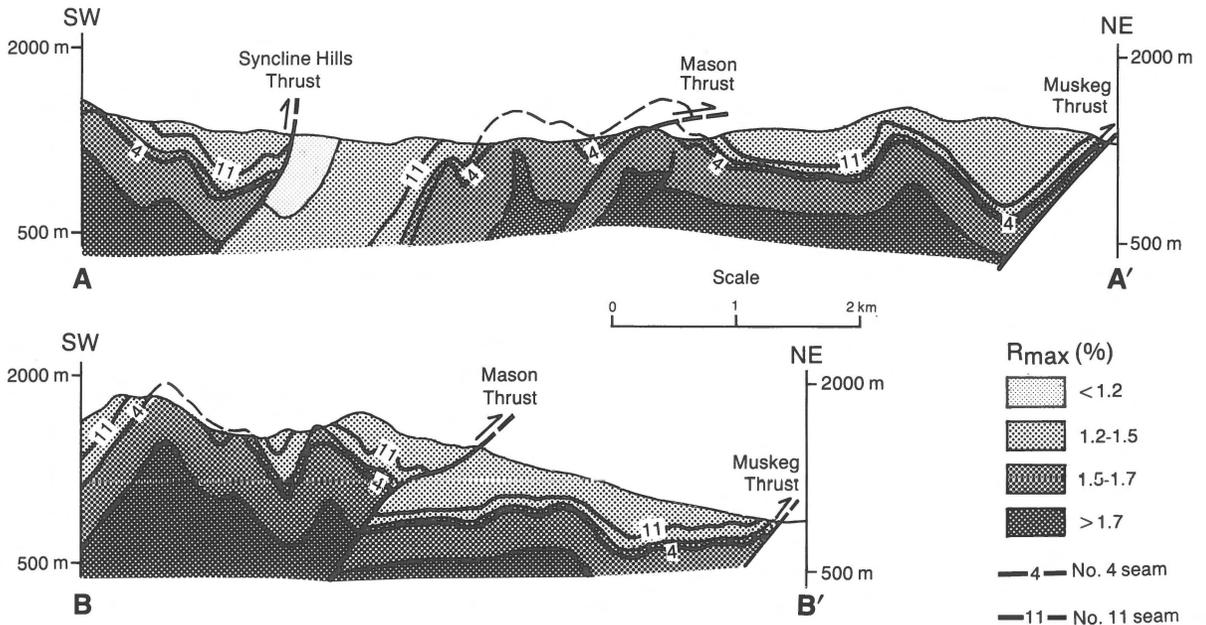
Fig. 5. Cross sections showing relationship of coal rank to deformed strata. The section lines AA' and BB' are indicated on Figs 1 and 4. Modified from Kalkreuth & Langenberg (1986).
