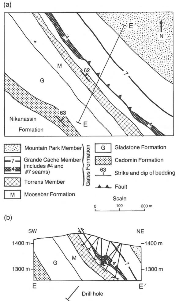
Fig. 9. Geological map (a) and cross section EE' (b) of part of the No. 12 Mine area. The cross section, which is based on eight drill holes, illustrates the presence of a duplex in the No. 4 coal seam.
