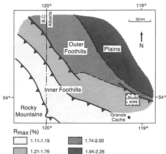
Fig. 3. Maximum vitrinite reflectance variations for coal samples from the Gates Formation in the area north of Grande Cache. Data for Plains and Outer Foothills are from subsurface samples (core and/or cuttings), while data for Inner Foothills come from outcrop samples. The location of the area shown in Fig. 1 is indicated. Modified from Kalkreuth & McMechan (1984).
