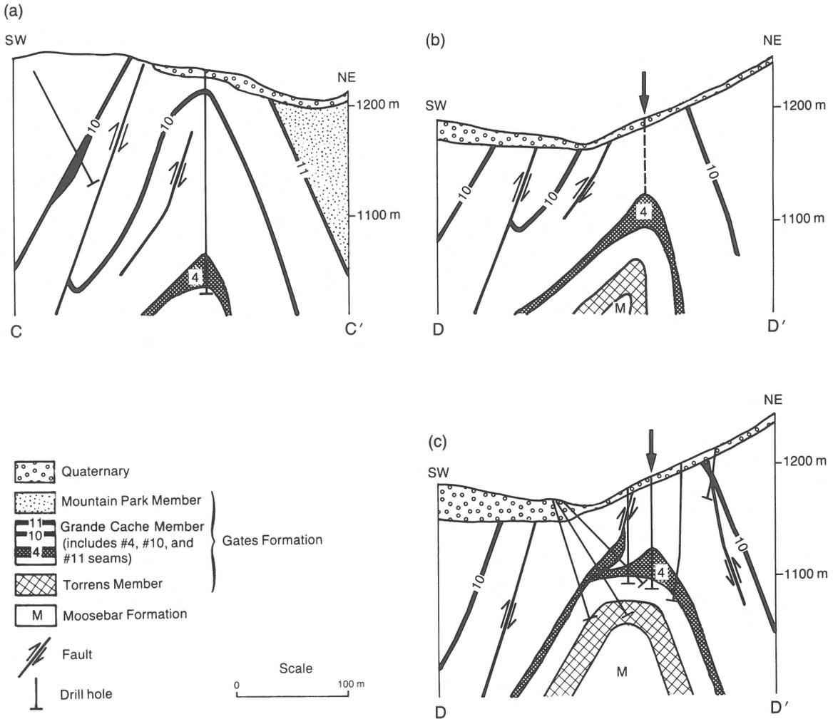
Fig. 8. Cross sections through the South Pit area. The lines of section are shown on Fig. 7. (a) Section CC' based on outcrop mapping and two drill holes. (b) Section DD' as predicted from Section CC'. The location of the first drill hole to test the structure is indicated with an arrow. (c) Section DD' based on seven drill holes.
