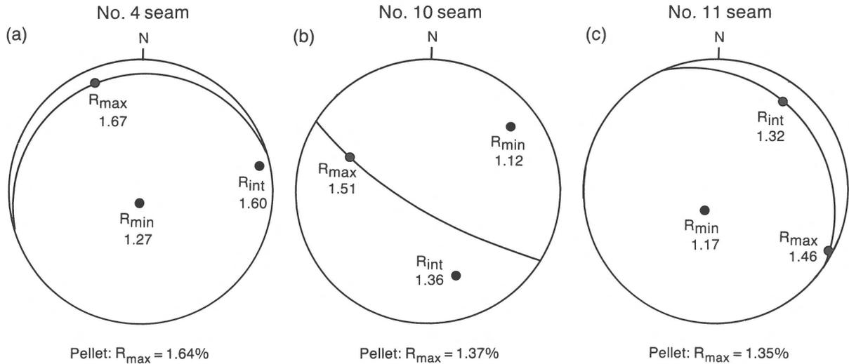
Fig. 6. Orientations and magnitudes (percent reflectance) of principal reflectance axes of vitrinite for samples from (a) No. 4 seam, (b) No. 10 seam and (c) No. 11 seam. The orientation of the bedding plane is indicated by the solid curve. The magnitudes of maximum reflectance of vitrinite as determined on pellets made of crushed coal particles of these samples are also shown.
