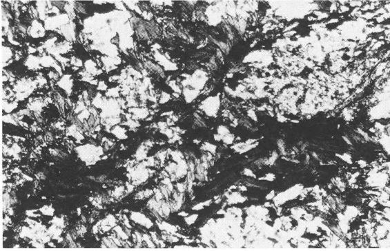
Fig. 16. Microphotograph of biotitization affecting felsic metavolcanite, 300 m NW of lake Älvlången. Deformed and recrystallized biotite occurs along fractures and network veins. This type of alteration occurs locally, and is related to the phlogopite veining in the footwall marbles. Plane polarized light. Field of view is 3 \times 2 mm.
