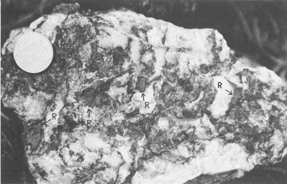
Fig. 9. Hydrothermal marble breccia in the footwall of the ore zone. Note the irregular and subrounded marble fragments (white), and the smaller rhyolitic fragments (grey, arrow with R).
