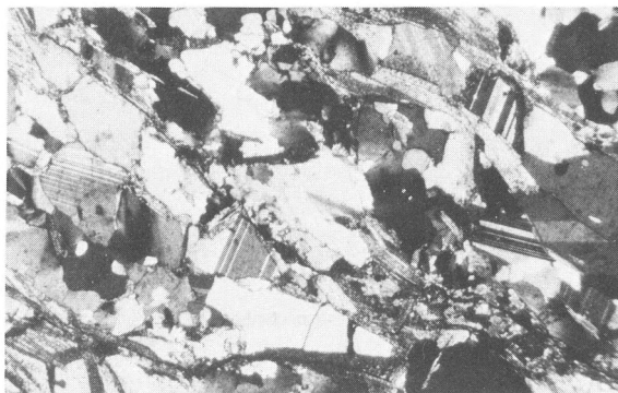
Fig. 14. Microphotograph of albitized felsic metavolcanite, 1 km N of Kopparskallen. The foliation is expressed by elongate, undulose quartz grains (white) and a parallel orientation of partly recrystallized muscovite flakes (grey). This type of alteration occurs regionally, and is presumably not directly related to the ore-forming processes. Note the coarse-grained fabric relative to the microclinized equivalent in Fig. 15. Plane polarized light. Field of view is 3 \times 2 mm.
