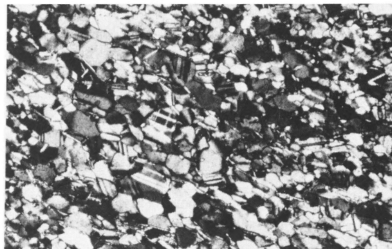
Fig. 15. Microphotograph of microclinized felsic metavolcanite, 300 m N of Kopparskallen. This type of alteration occurs regionally, and is presumably not directly related to the ore-forming processes. Note that the fabric is less well recrystallized and finer grained than the albitized equivalent in Fig. 14. Plane polarized light. Field of view is 3 \times 2 mm.
