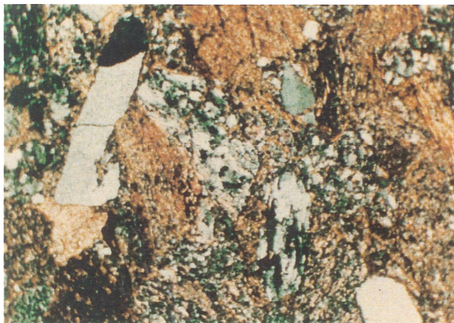
C. Westphalian D (Aguiró Fm.), coarse-grained, highly immature sandstone. Grains are mostly phyllite and micaceous quartzite ('recycled orogen'). No. 6 in table 1.
