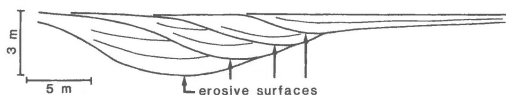
Fig. 12. Vertical and lateral aggradation body. The channel deposit consists of several units with erosive base: the units are obliquely arranged within the main channel.
