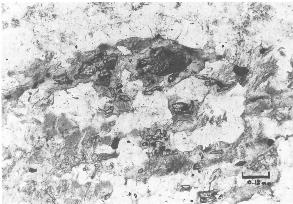
Fig. 3d. Corundum (high relief) in partly chloritized biotite (greyish). The two biggest crystals enclose spinel (dark grey, almost opaque in photograph). Note the presence of minute crystals of an opaque mineral and tiny needles of sillimanite. Amoa-El Barquero Granite from the contact aureole of the Estaca de Bares Granite.
