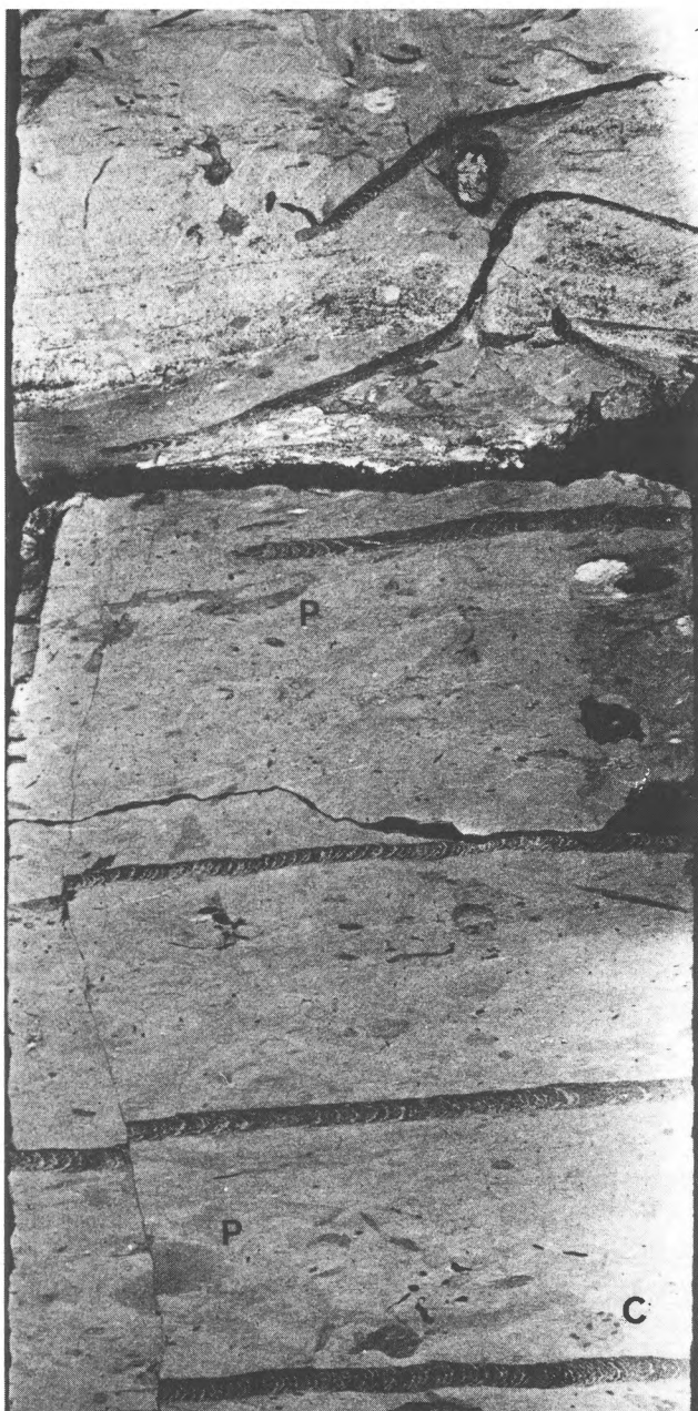
Fig. 13 Zoophycos showing gradually larger burrow-tube diameter down through the section. Note the presence of other trace fossils Chondrites (C) and Planolites (P), and the general biomottled appearance. Core from T-1 at 7269' (BKB), core diameter 10 cm.
