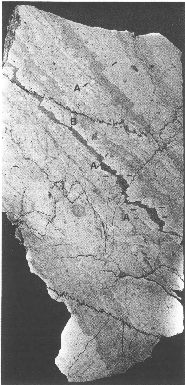
Fig. 10 Shredded structure in flow-induced lamination. Shredding is small-scale folding and microfaulting (A). Small light-coloured chalk intraclasts are present in the matrix (B). Core from T-1 at 7535' (BKB), core diameter 10 cm.
