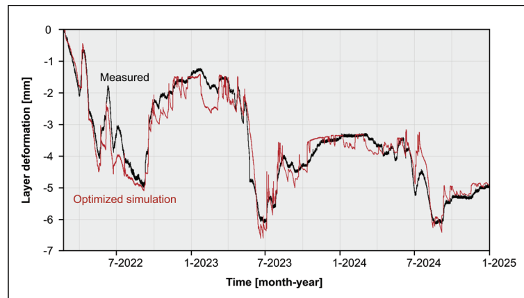
Figure 10. Comparison between the Briaud model results optimised seasonally and measurements for Site 1, Hazerswoude.
