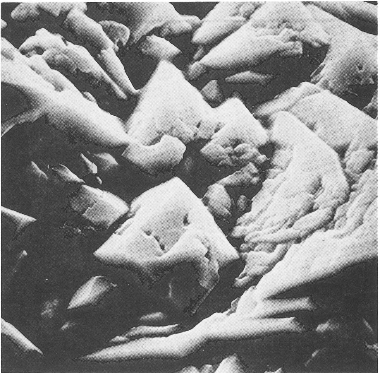
Fig. 2 Scanning electron micrograph of rhomboclase (synthetic). 3500 x, TFDL 340-3
