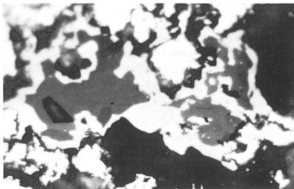
Photo 6 Rickardite (medium grey), surrounded by weissite (light grey) and melonite (white). Mindola Mine. Magnification 300 x.
