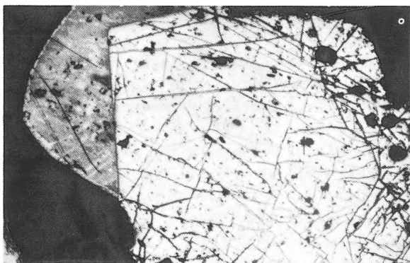
Photo 2 Subhedral carrollite veined by digenite and surrounded by bornite (medium grey). Nchanga Mine. Magnification 250 x.
