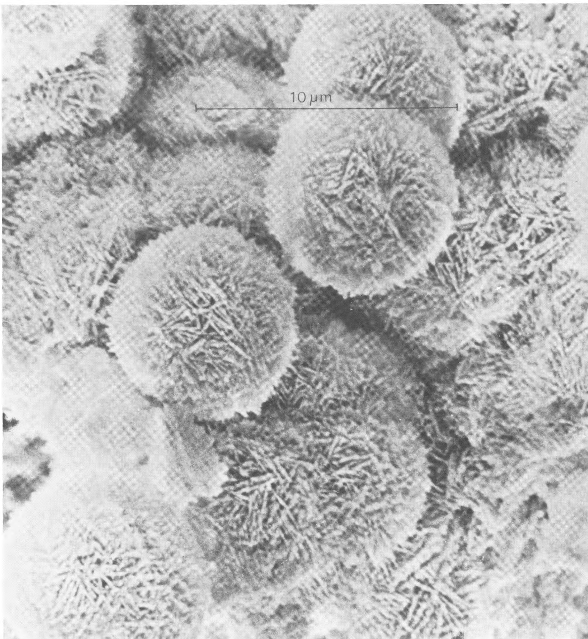
Fig. 16 Scanning electron photograph of sample 110, showing botryoidal structures with a crystalline surface. Magnification 7200X. T.F.D.L. Wageningen.
