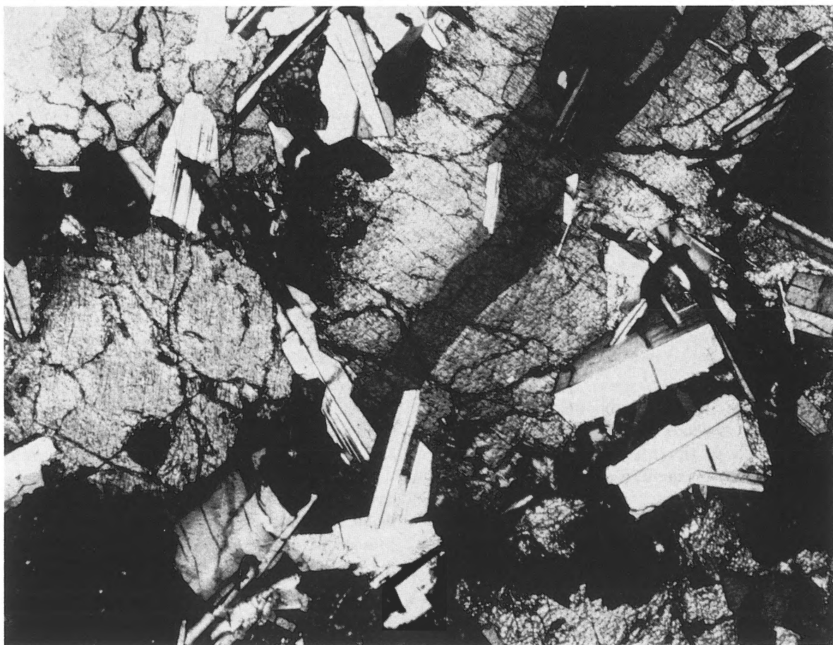
Fig. 4 Thin section (Apollo II; 10044) between crossed polars showing sub-grain misorientation in pyroxene grain. The largest grain of pyroxene has a dark band down the middle; the central sub-grain is very near extinction while the outer regions appear bright. Ilmenite, plagioclase feldspar and a small area of cristobalite can also be seen (X 50).
