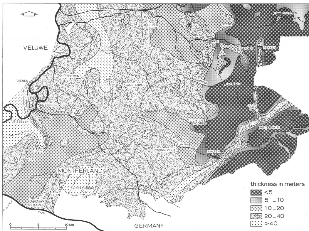
Fig. 4 Isopach map of the water-bearing layers, comprising the Kreftenheye, Drente and the Urk formations.
